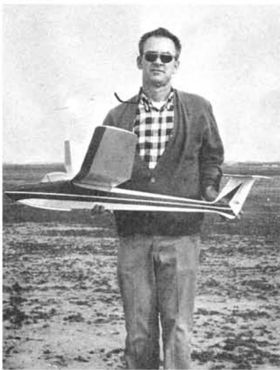
Nose to the grindstone. (Ooooh, that's awful!) Fuselage balanced to display inner space area. Servo installation comes next, then top sheet.
